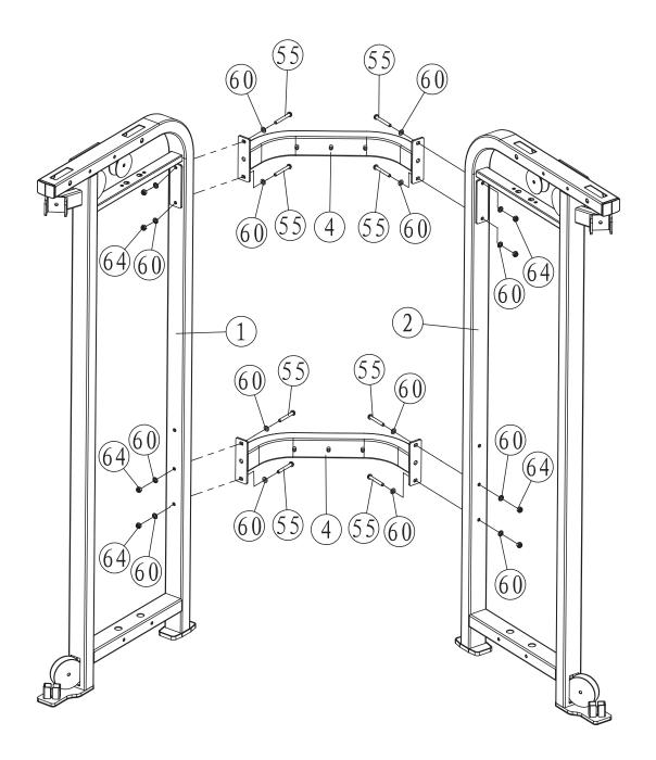
STEP 1 Connect Left Frame (1) and Right Frame (2) with the two Rear Beams (4) using Bolts M10X80 (55), Washers M10 (60), and Nylon Nuts M10 (64).
